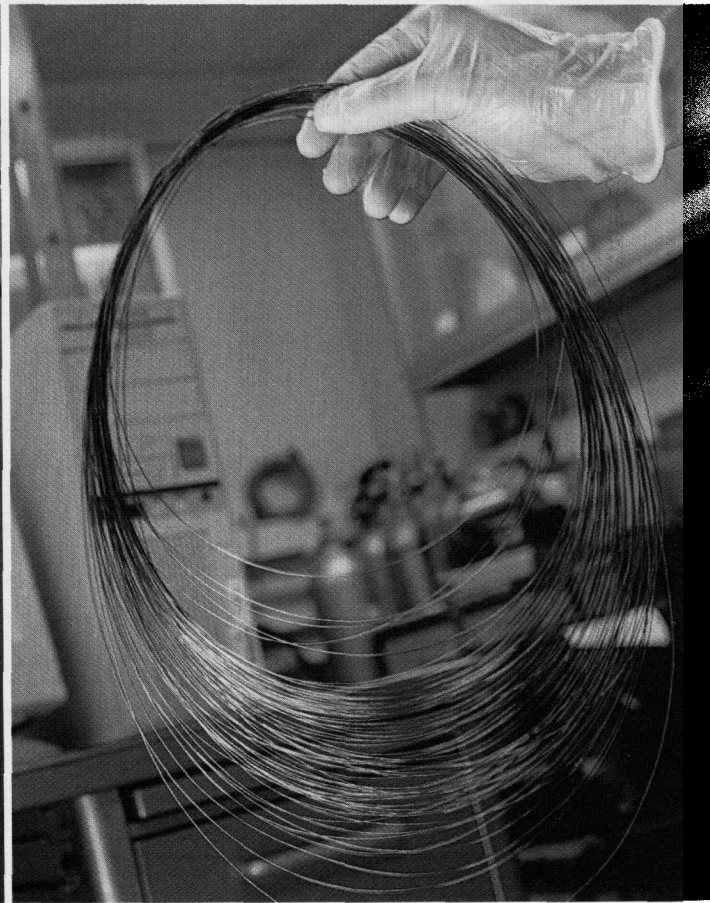
From rod to thread: In Yoel Fink's lab, centimeter-scale rods are thinned as they are pulled through a furnace known as a "draw tower" (top left and right). The process, which is monitored on a control unit (bottom left), produces optical threads just 400 micrometers in diameter (bottom right). PHOTOGRAPHS BY WEBB CHAPPELL
